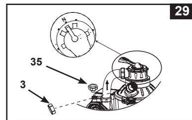
**IMPORTANT: To prevent damage to the 6-way valve, always depress the valve handle before turning. Always switch off pump before changing the 6-way valve position.**
