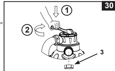
5. Switch off the pump, change the 6-way valve to "RINSE" position (see drawing 25).
