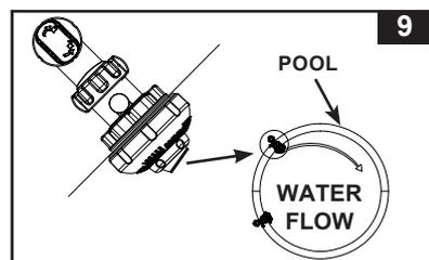
**NOTE:** Do not cover the air jet valve (15) with the valve cap (34) under normal situation or when the pump is operating. See Troubleshooting Guide section for more details.
