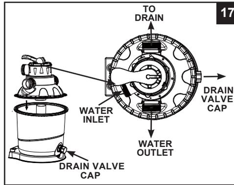
**IMPORTANT:** There are three hose connection ports on the 6-way valve, ensure the outlet connection (from filter to the pool) on the valve is facing towards the pool (see drawing 18).
