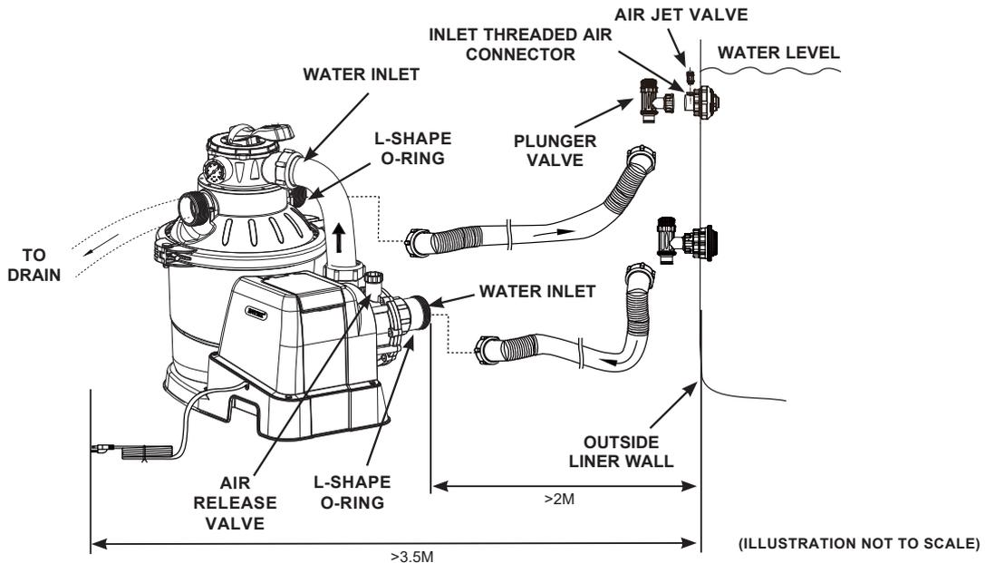
According to the International Standard, IEC 60364-7-702, on electrical installation of swimming pools and other basins equipment, the following installation distances must be respected:
