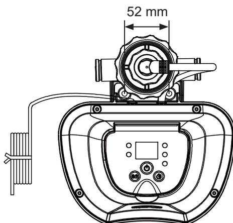
1. The mounting holes are 6.4 mm in diameter and spaced 52 mm apart.
