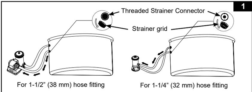
2. Screw the hose adaptor (4) to the threaded strainer connector, from inside of the pool. See Fig. 2.
