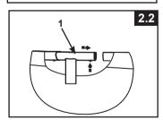
The last joint connection may be difficult to complete, but can be easily done by simultaneously raising this last joint and beam more than 2 inches (5 cm), and connect the beam to the joint while lowering these pieces to their normal position. The joint will slide into the beam (see drawing 2.3). Make sure the last joint is fully assembled before proceeding to assembling the legs.
