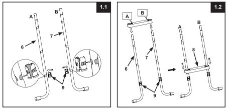
**IMPORTANT:** Ensure the J-shaped legs are pointing outwards before installing the steps.
