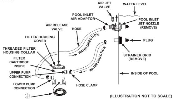
The power cord plug to the 220-240 volt electrical power source of the filter pump must be positioned more than 3.5 m away from the pool walls. Check your local authorities to determine the appropriate standard and requirements for "electrical installation of swimming pools and basins equipment". The following table is for reference only:
